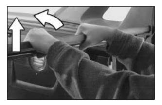
Remove the front rail by first twisting up the edge nearest you, to clear the midgate seals, and then pulling it out from the side rails.
